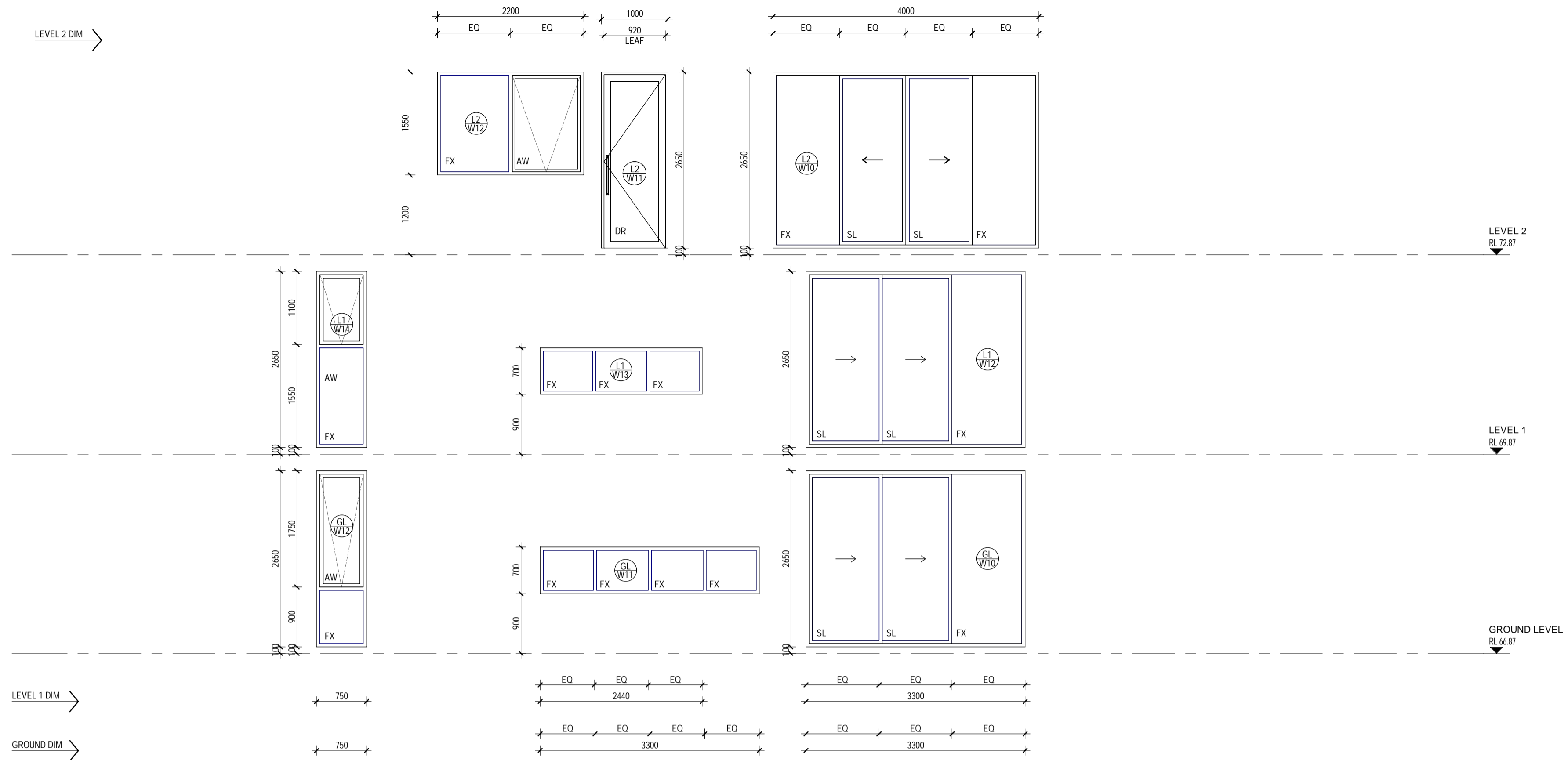
01 WINDOW SCHEDULE - EAST ELEVATION A900 SCALE 1 : 50
