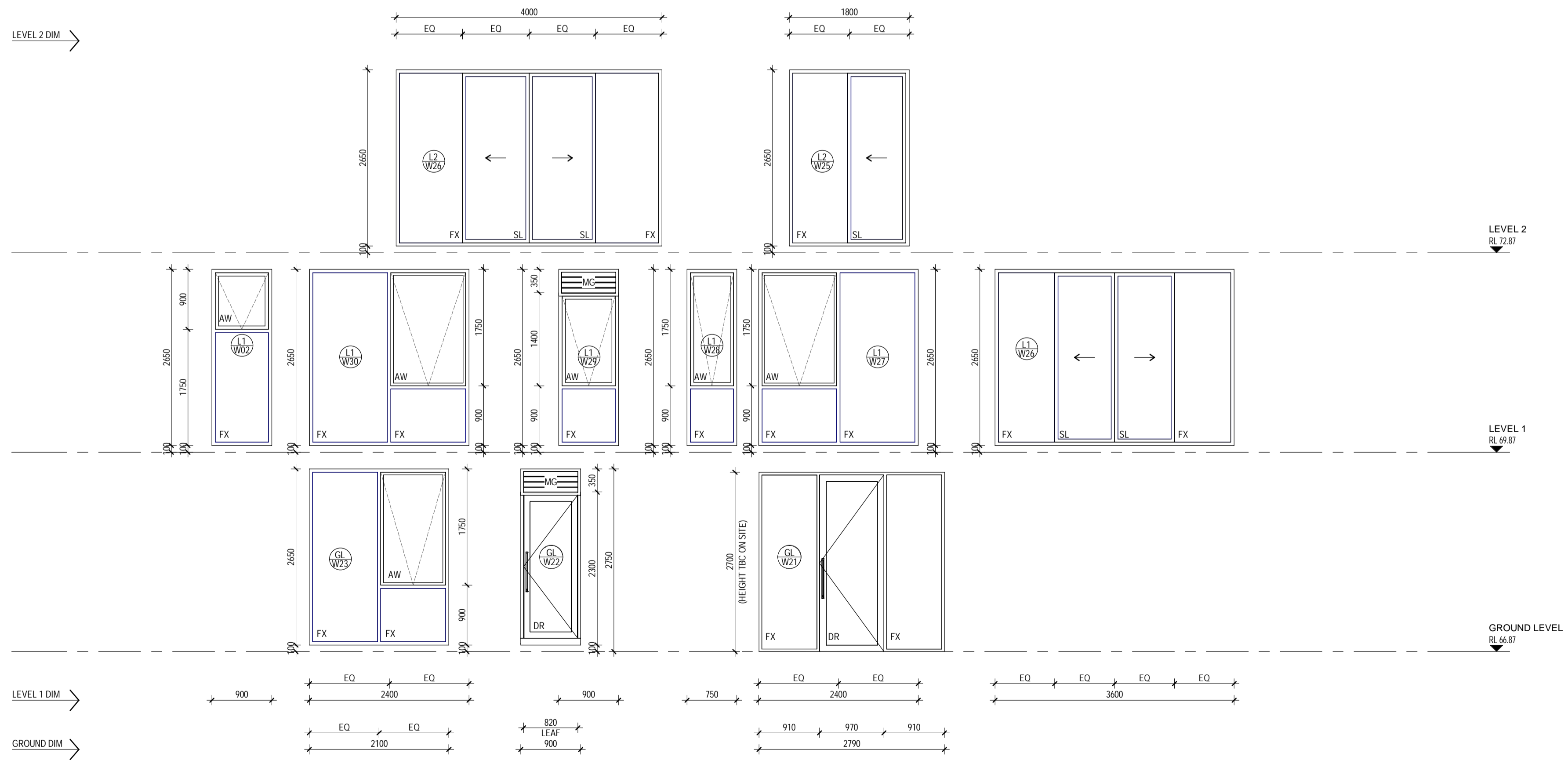
02 WINDOW SCHEDULE - WEST ELEVATION A900 SCALE 1 : 50
