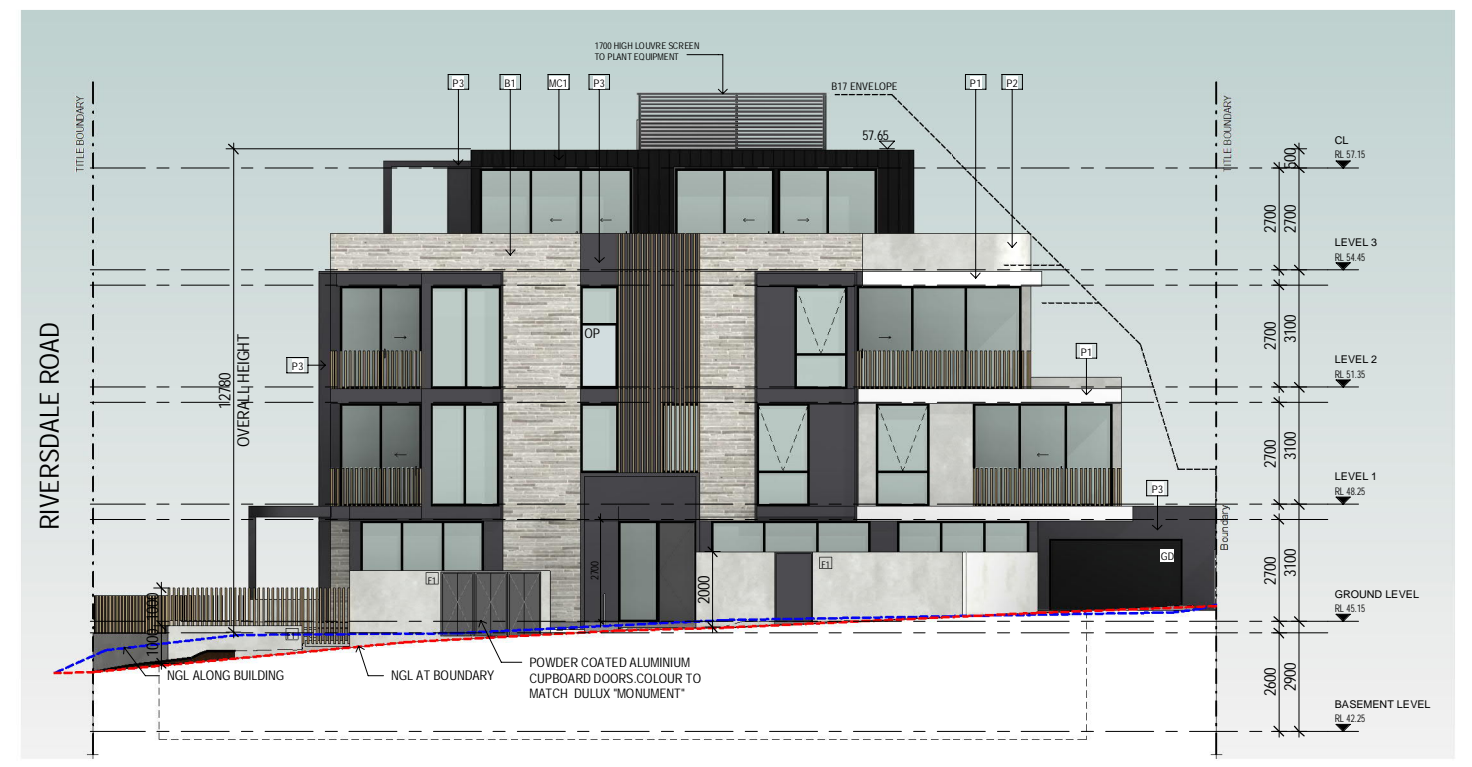
2 WEST ELEVATION - HASTINGS RD TP200 SCALE 1 : 100
